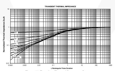
Figure 11. Transient Thermal Response Curve.
