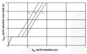
Figure 7. Gate Charge Characteristics
