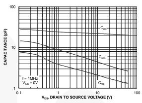
Figure 8. Capacitance Characteristics
