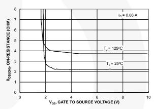
Figure 3. On-Resistance Variation with Temperature
